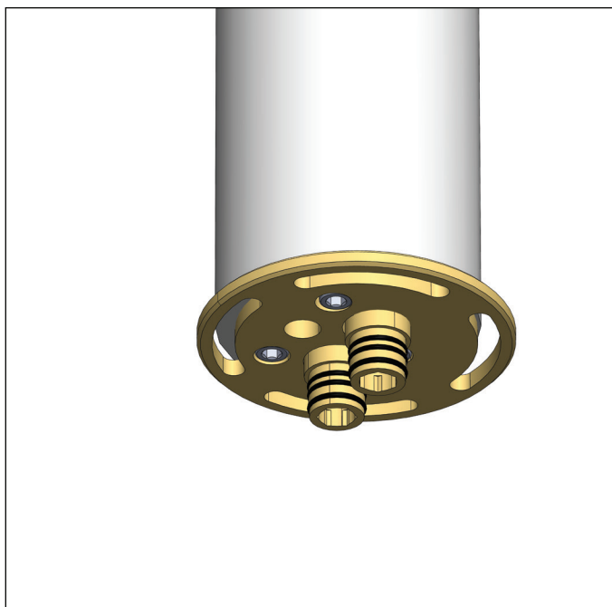
Ensure double o-rings are undamaged and greased
